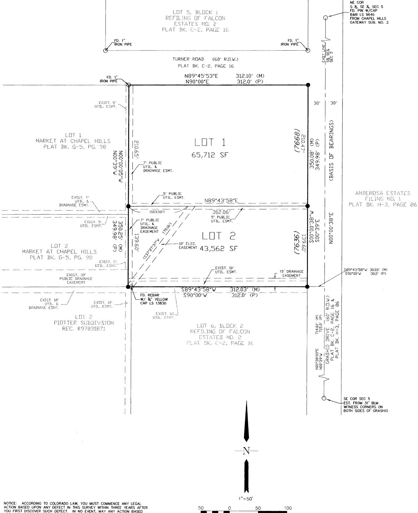
LEGEND FOUND MONUMENT AS NOTED SET #4 REBAR W/CAP PLS 24964 EASEMENT SECTION LINE (7668) ADDRESS PLATTED DIMENSIONS N90°00'E 312.0 (P) MEASURED DIMENSIONS N89'45'53"E 312.10' (M) (S37\*27'37"W 170.16') EASEMENT DIMENSIONS
